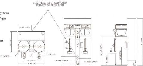
Water Requirements: 20-75 psig, 1.25 gpm flow rate. Water inlet is 3/8 Male Flare Tank Capacity: 7.6 gallons
